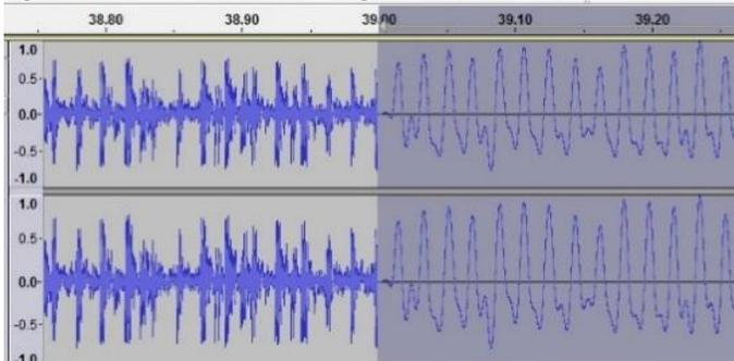
**Figure 10: THE SOUND OF THE ENGINE BEFORE AND AFTER FILTERING**
