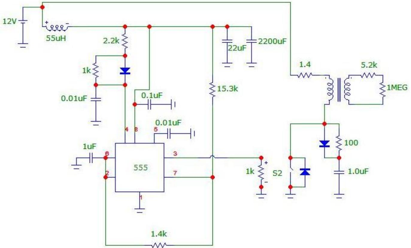
Figure 2 THE IGNITION CIRCUIT DIAGRAM
