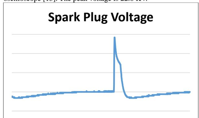
Figure 9: MEASURED SPARK PLUG VOLTAGE
