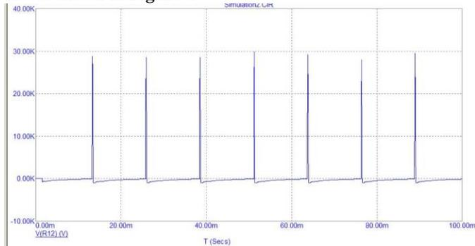
**Figure 4: SIMULATION SPARK PLUG VOLTAGE**
