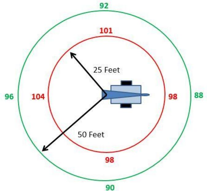
Figure 8: ENGINE SOUND FIELD ON VAPOR
